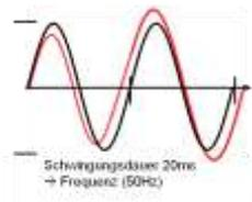
The oscillation of alternating current in the German electricity grid
